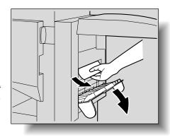
11 If the paper could not be removed in step 10, turn the misfeed-clearing dial in the folding section clockwise.
